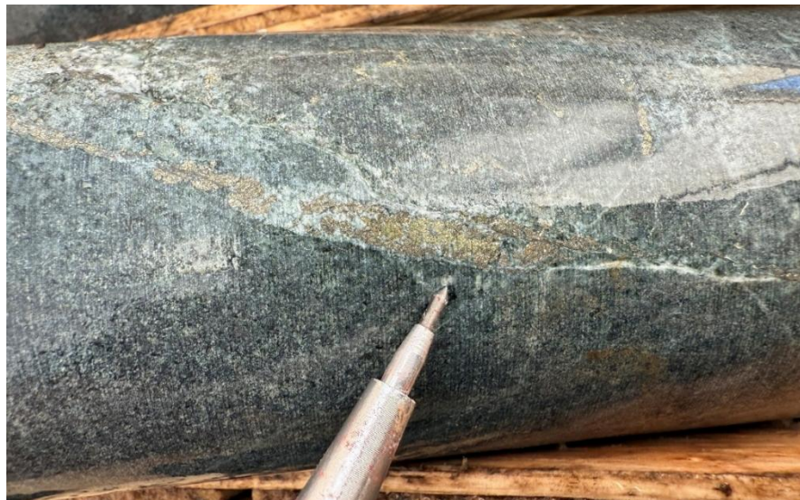
Figure 3 – Diorite with quartz-pyrite-chalcopyrite veining at 51.7m in hole AZ25-004.
