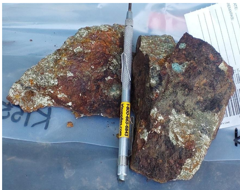
Figure 6 – Sample K155456 from the AZ Skarn occurrence, grading 26.7% Cu and 1.84 g/t Au .
