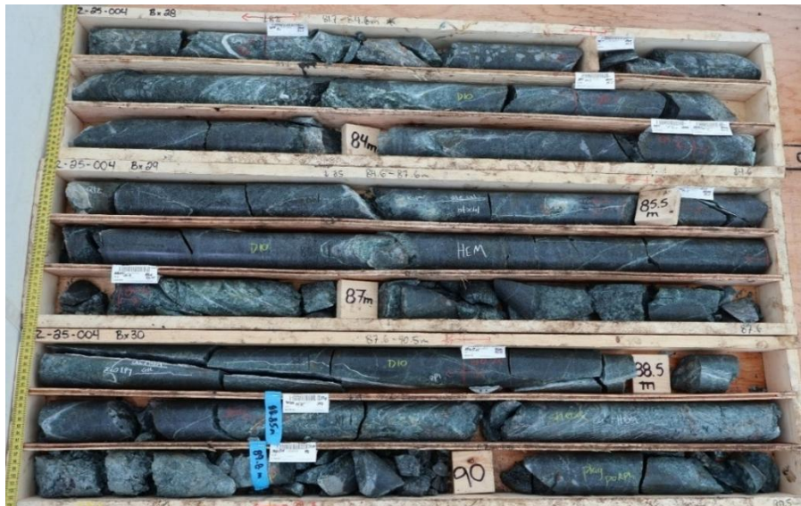
Figure 2 – Altered diorite intersected in AZ25-004 located at the New Target Zone. Partially hematized magnetite visible along with disseminated and veined pyrite-minor chalcocopyrite throughout.
