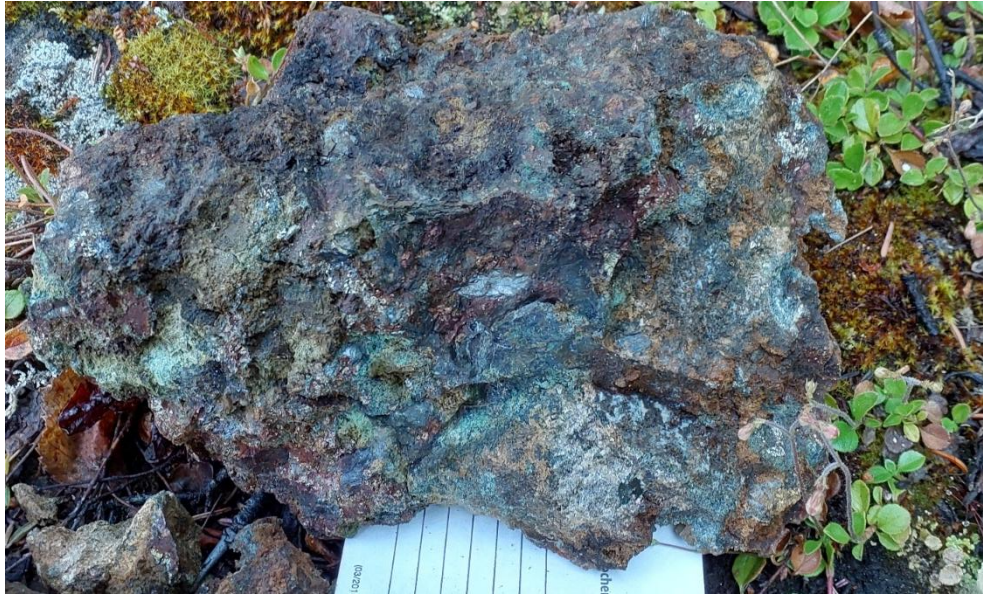
Figure 7 – Sample K140142 from the AZ skarn occurrence, grading 6.7% Cu and 5.11 g/t Au .
