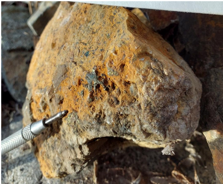
Figure 8 – Float sample K155003 of oxidized vein found in a new area in the central part of the AZ claim block, grading 2.16 % Cu and 4.95 g/t Au .
