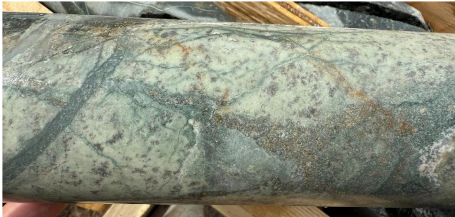
Figure 1 – Altered diorite with pyrite and chalcocopyrite in veining and disseminated, from AZ25-004 at 135 metres.
