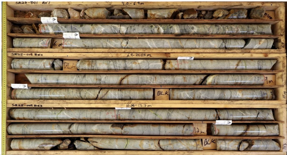
Figure 5 - Top of first hole, SR25-001 at Star River in quartzite unit with pervasive pyrite-arsenopyrite-galena veinlets.
