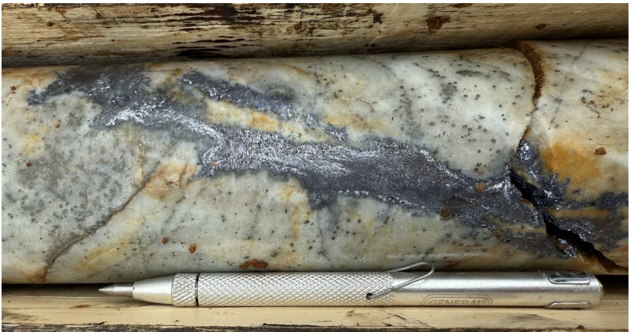
Figure 1 - Hole SR25-003 at 18m showing galena vein cutting quartzite with disseminated pyrite-arsenopyrite.
