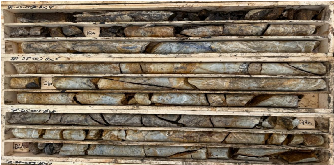
Figure 4 - Veined and oxidized quartzite at the top of hole SR25-003 in the F2 zone. Galena, pyrite and arsenopyrite are present in quartz-ankerite veins.
