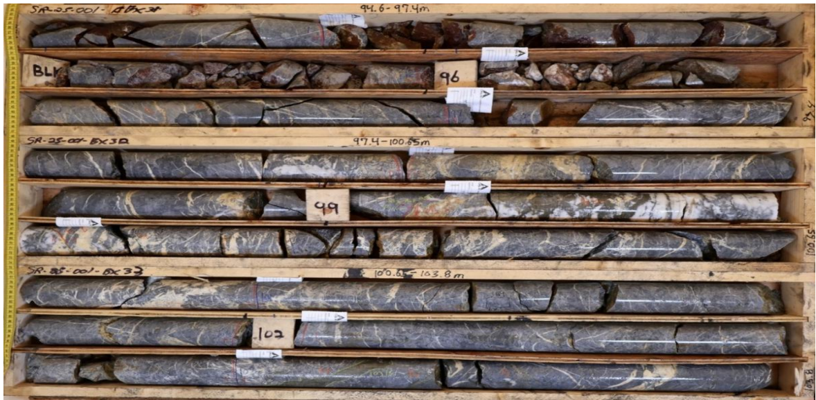
Figure 6 - Vein zone around 100m in SR25-001 consisting of a swarm of quartz-ankerite-pyrite-galena veins hosted in silicified sediments.
