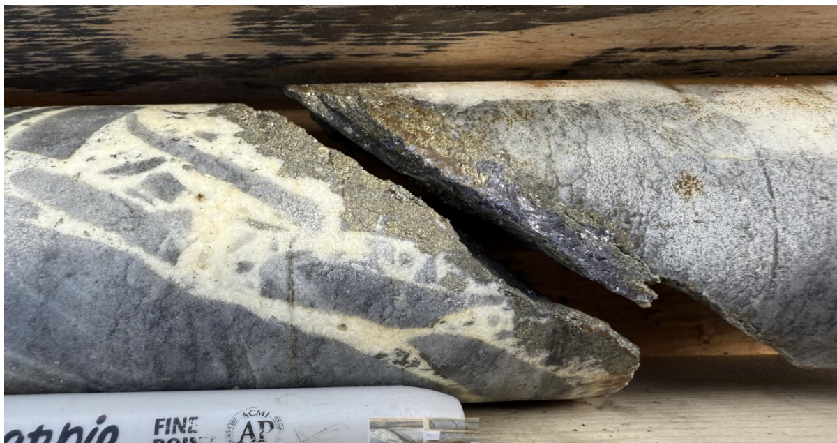
Figure 3 - SR25-002, Brecciated galena-pyrite-ankerite-quartz vein zone at 36m, hosted in a dolostone unit.
