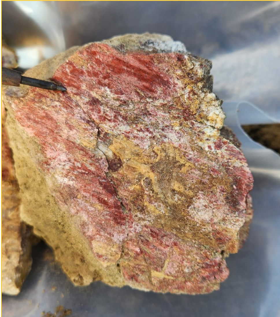
Figure 3- Sample K140214 showing intensely hematite-altered basalt with quartz-calcite stringers. Contains 111.5 ppm Cu.
