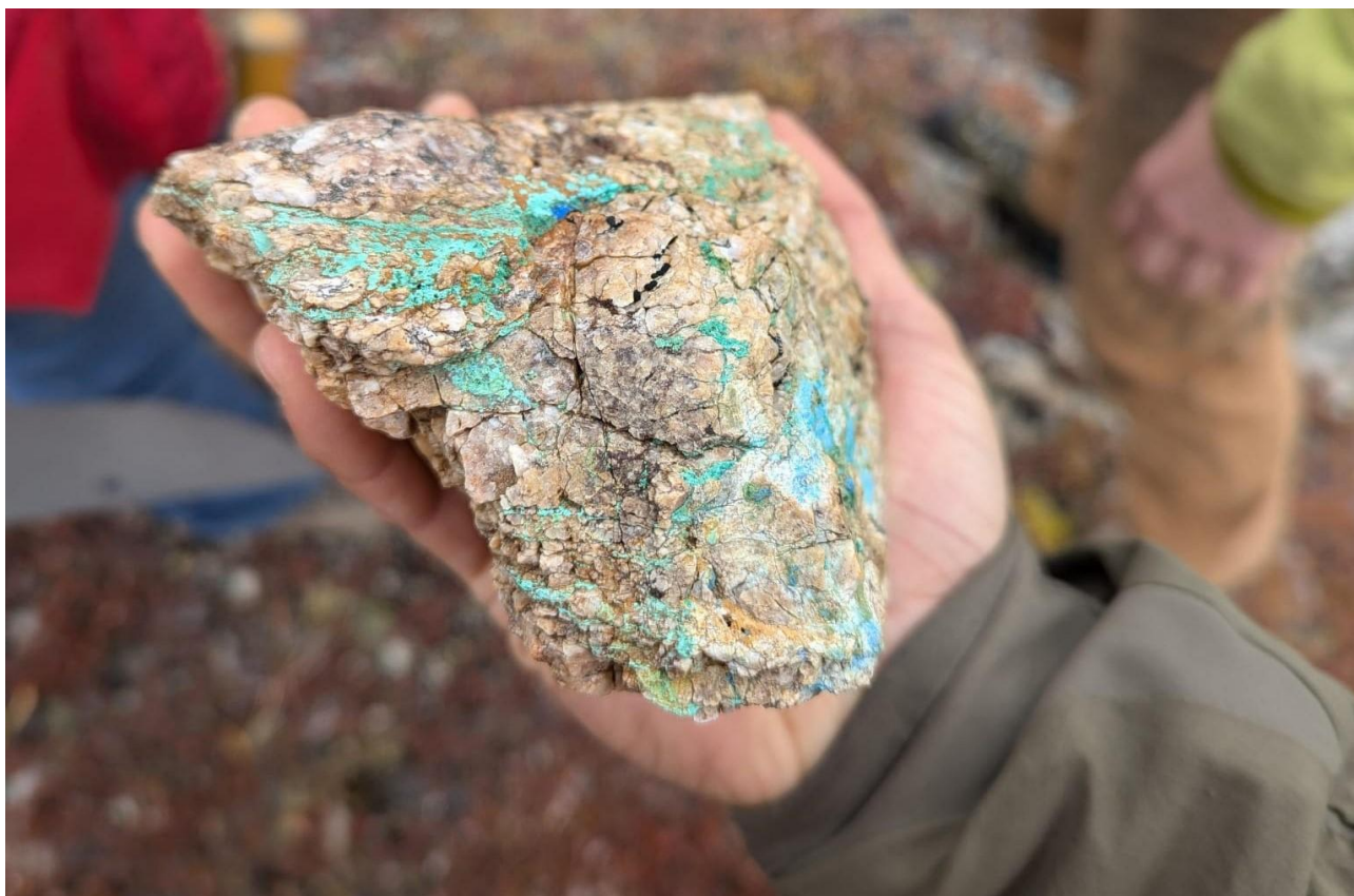
Figure 2- Sample K140202 Grading 3.49% Cu
