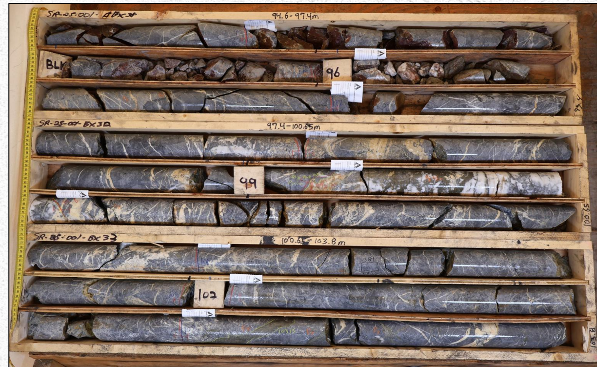
VEIN ZONE IN SR25-001 CONSISTING OF A SWARM OF QUARTZ-ANKERITE-PYRITE-GALENA VEINS HOSTED IN SILICIFIED SEDIMENTS.
