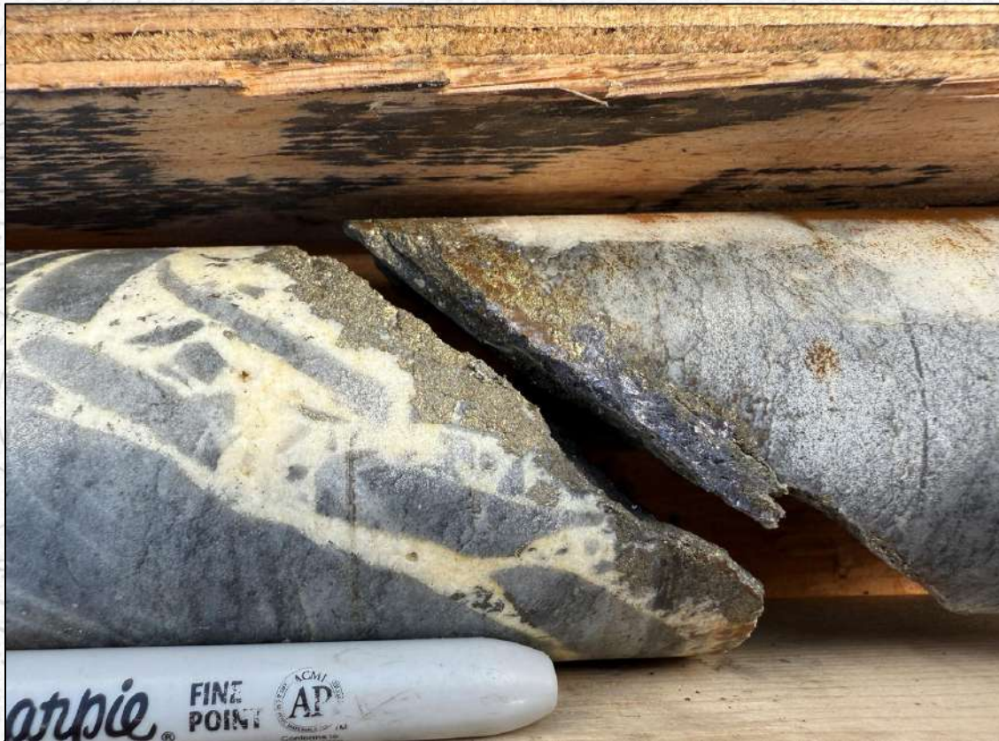
HOLE SR25-002 AT 36M SHOWING GALENA-PYRITE-ANKERITE-QUARTZ IN VEIN ZONE WITHIN SILICIFIED SEDIMENTS.
