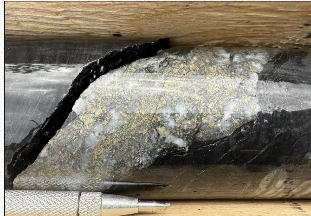
SR25-003, PYRITE-QUARTZ-MINOR ARSENOPYRITE VEIN AT 140M HOSTED IN SILICIFIED PHYLLITE UNIT.
